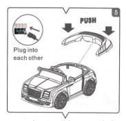
6. Installing the Rear Spoiler: Locate the wire at the bottom of the rear spoiler. Feed the wire through the open slot at the top of the rear of the car and connect the wire to any of the 4 white slots located on the white power board. Once connected place spoiler tabs into the open slots at the rear of the car and push until you hear a click.
