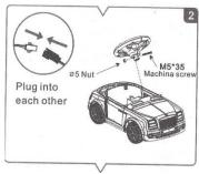
3. Installing Steering Wheel: Locate the music/horn wire at the end of the steering wheel, and connect it to the power wire located on the steering rod. Once wires are connected, remove screw and nut located on the steering wheel column. Once screw and nut are removed, align hole on steering column with the hole located on the steering rod. Insert screw through the hole, followed by tightening the screw to the nut until tight.
