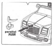
Hood Ornament: Insert the tabs located at the bottom of the hood ornament into the slots located at the front of the vehicle hood.
