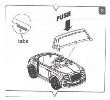
4. **Windshield Installation:** To install the windshield into the body of the car, align the tabs located at the bottom of the windshield with the holes located above the dash board at the front of the car. Insert tabs into the holes, and push down until you hear a click.
