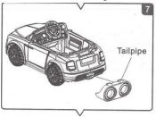
8. **Installing the Tailpipe:** Fit the tailpipe into the slots located at the bottom rear of the vehicle body. Push the tailpipe into the slot until you hear a click.
