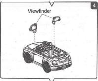
Installing Rearview Mirrors: Fit the tabs on the bottom of the Rearview Mirrors
