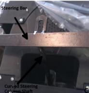
Rotate the axle that is still connected to steering bar, toward the front of the car. You will need to slightly bend steering bar over the curved steering column shaft to get completely rotated. (See Image C)
