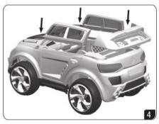
1. Install the car windows, rear windows, and rear speaker deck: Snap rear speaker deck into place at the rear of the car. Snap rear window into place and secure with screws from the bottom of the car. Snap door window into place on the upper part of the door and secure with 5 screws. Repeat steps for both door windows.
