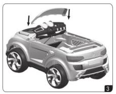
5. Install Gauges and Windshield: Match color of electrical connector on gauges to corresponding electrical connector on the dash and make connection. Snap gauge into place on the dash. Repeat steps for 2<sup>nd</sup> gauge. Insert the windshield to proper location on the front of the dash area. Snap into place and secure with 2 screws.
