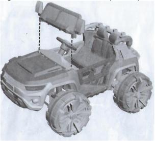
Align the windshield with the vehicle & push into place.
