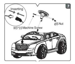
5. **Install Steering Wheel:** Connect electrical connection between the steering wheel and the wires from the car. Slide steering wheel onto the steering shaft. Align the screw hole in the steering shaft and the steering wheel and slide the bolt through the hole. Apply the nut to the end of the bolt and tighten until snug. See Fig. 7
