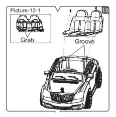
Install the Seat: Slip tabs on back of seat into the slots in the body of the car. Attach seat to body through the two holes located in the front corners of the seat with 2 screws. See Fig. 10
