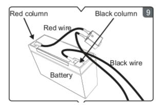
6. Connecting the Battery: Slide red wire with spade terminal onto the red or positive side of the battery. Slide the black wire with spade terminal onto the black or negative side of the battery. DO NOT INSERT THE RED WIRE ONTO THE BLACK OR NEGATIVE SIDE OF THE BATTERY! See Fig. 9
