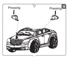
4. **Install exterior mirrors:** Place mirrors into place on the body press firmly until a clicking sound is heard. (Letting you know they have snapped into place.) See Fig. 6
